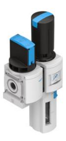
Consisting of manual on-off valve including silencer, filter regulator and wall mounting plate. 12 bar maximum output pressure, 40 µm filter, with pressure gauge, lockable regulator head, plastic bowl with plastic bowl guard, manual condensate drain, direction of flow: from left to right.
